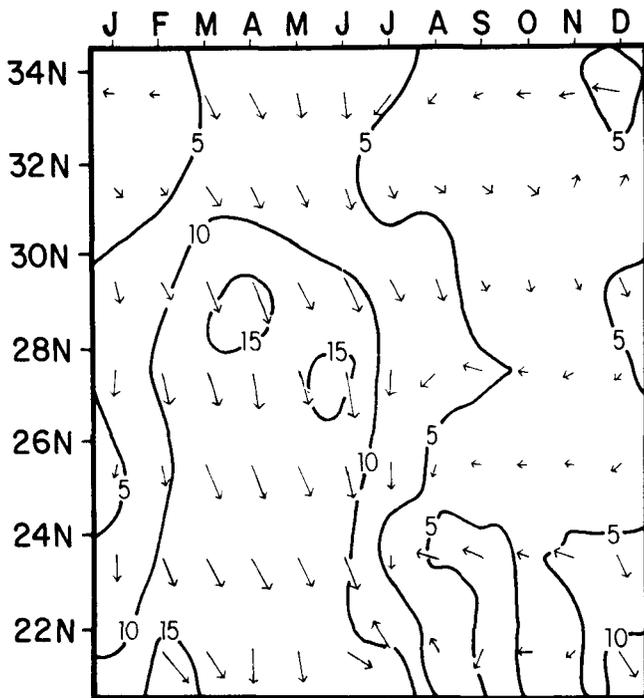
FIGURE 7. Seasonal cycle of ship drift near the coast. Resultant vector were summarized by month from the NAVOCEANO ship drift file, for a group of 2 degree squares along the coast from latitude 20°N to 34°N. Units are cm/sec. Magnitudes are contoured at intervals of 5 cm/sec. Vector symbols are scaled according to the key in Figure 9A.
