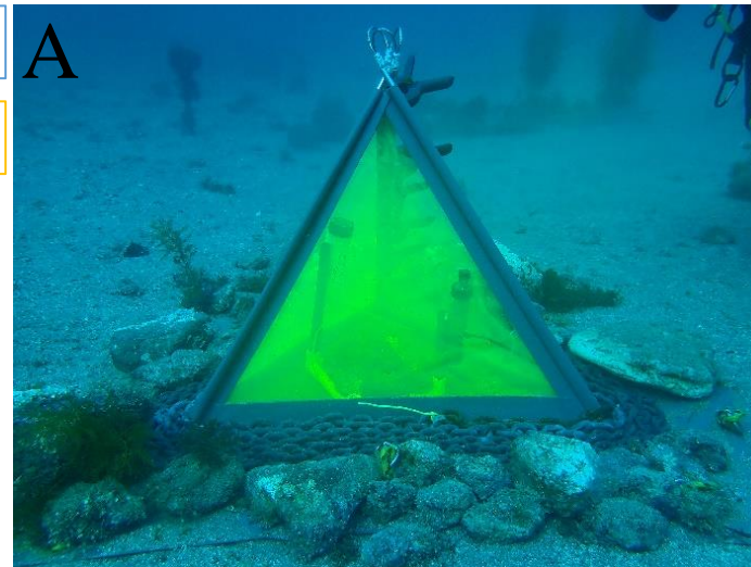
Fig. 2 A) Chamber isolating injected seawater with dye indicator added to locate seawater leakage. B) Identified source of leakage for future improvement.
